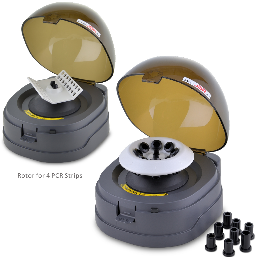
Rotor with 0.2ml, 0.5ml Tube Adaptors
